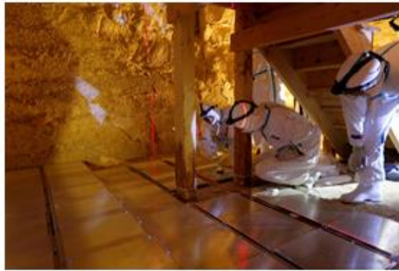
Muons Emulsion films setup in lower chamber
