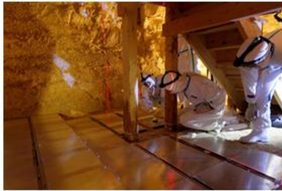
Muons Emulsion films setup in lower chamber
