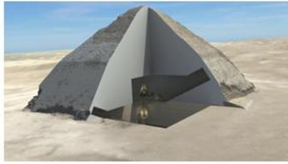
3D Cutaway view of Bent Pyramid with lower and upper chamber
